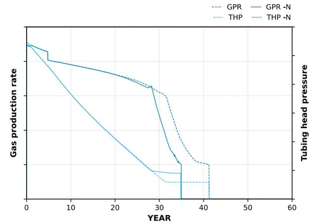
Gas production rate and tubing head pressure for a representative well.
